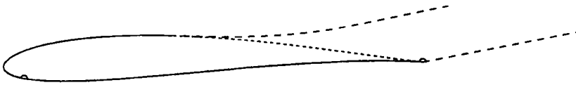
FIGURE 5. Separation streamlines in Joukowski-arc model, \alpha = 14^\circ , for the example of figure 4.
